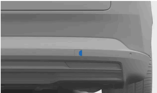
Rear towing eye fastening cover
