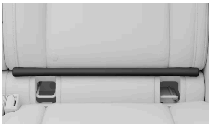
The folded ISOFIX flap, tucked into the gap above the anchorage points
