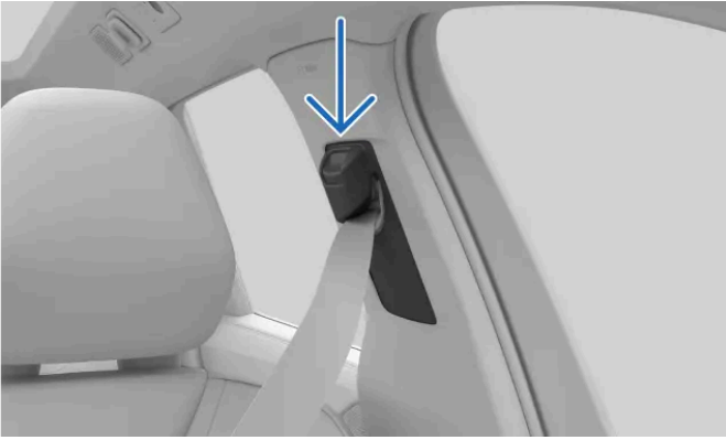
Seatbelt upper anchor point
