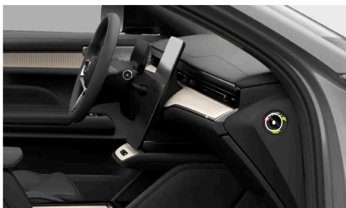
Location of the passenger airbag switch
