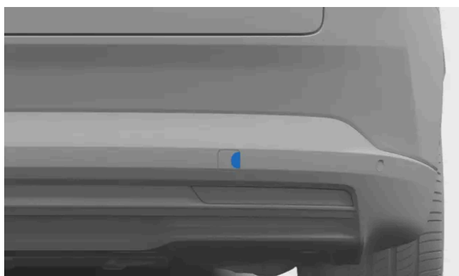
Rear towing eye fastening cover
