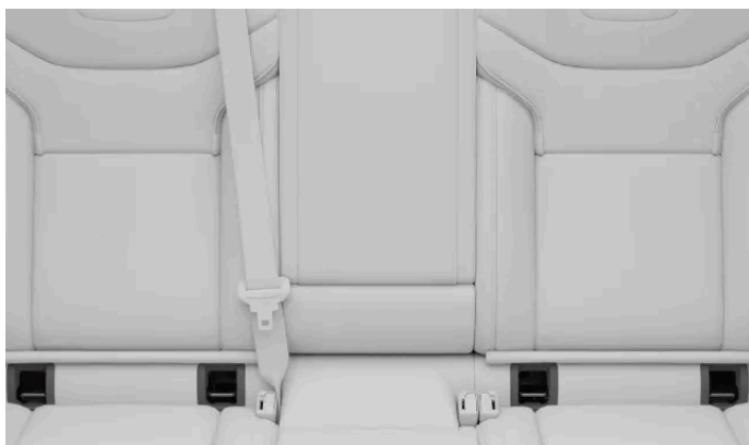
Locations of ISOFIX anchorage points for the rear seats
