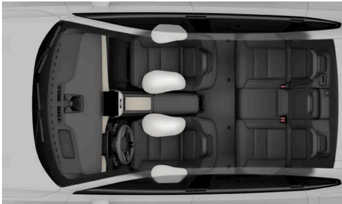
All side collision airbags for the front occupants.
