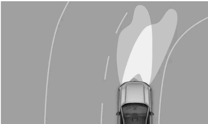
Typical function of the active bending lights.
