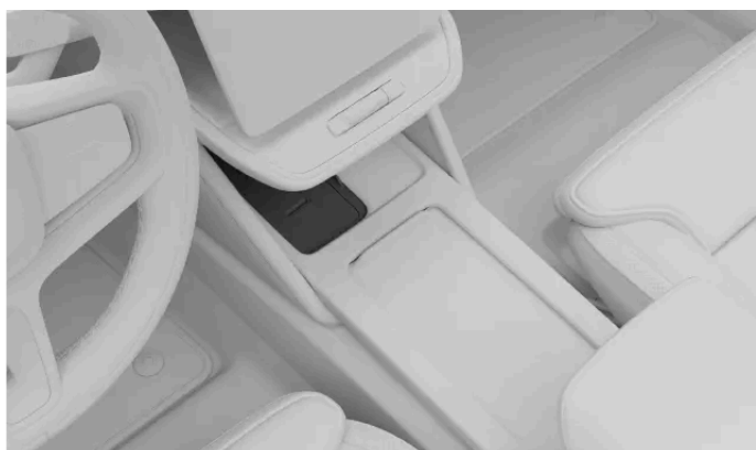
The card reader between the front seats is also the wireless charger.
