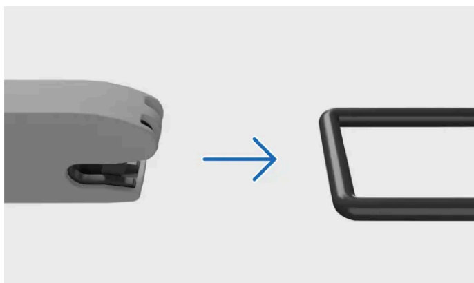
Attaching to ISOFIX anchorage point
