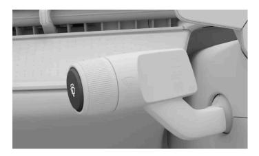
• Press and hold the button on the left-hand steering wheel stalk to activate the front washers.
