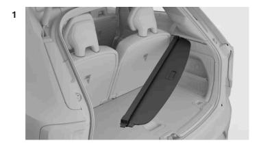
Put one end of the load cover into the indentation in the groove on one side of the boot. The indentation is highlighted with a marker line. Make sure that the end of the load cover lines up with the marker line.
