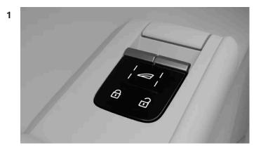
Press the window symbol at to switch between controlling the front and rear windows. The current window selection is indicated by the lights next to the symbol.
