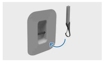
Fastening tether to top tether anchorage point
