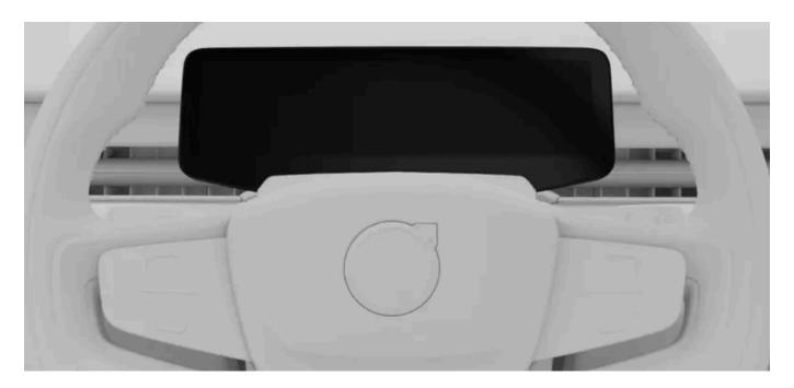
The driver display is located in front of the driver, behind the steering wheel. Its position changes along with the steering wheel when you adjust it to your preferred driving posture.
