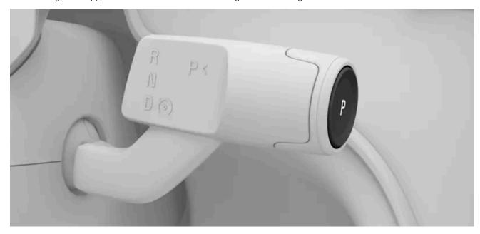
> The car transitions to a parked state, which includes engaging the parking brake. The new state is indicated in the driver display.
