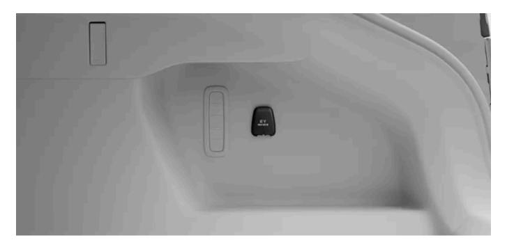
The 12 V electrical socket is on the right-hand side in the boot.
