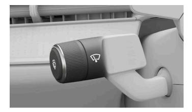
You can control the wipers and washers using the scroll wheel and button on the left-hand steering wheel stalk.
