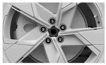
Tighten the wheel fasteners crosswise.
