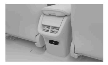
There are also two USB ports [1] in the rear part of the tunnel console.
