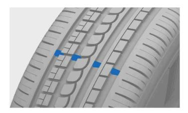
The narrow grooves that run lengthways across the tyre's tread pattern are tread wear indicators. On the side of the tyre are the letters TWI [1].
