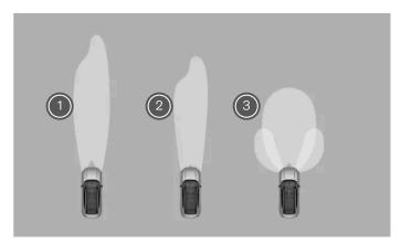
The passing beam has three automatic beam types
