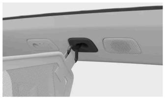
Fasten the lower corners of the net to the outer tether points behind the seats.
