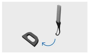
Fastening tether to lower tether anchorage point
