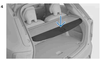
Tilt the outer edge of the load cover downwards so that it locks into position in the grooves.
