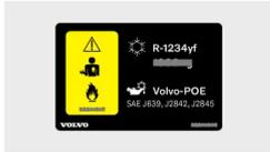
The label with information on climate system fluids is located on the underside of the bonnet.
