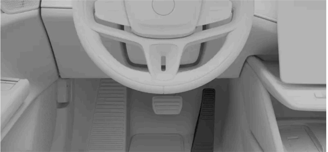
The braking behaviour changes through the use of the accelerator pedal. When you press the accelerator, the car accelerates as normal but releasing the pedal engages braking. The more you ease up on the pedal, the more braking action you get. By releasing the accelerator completely, you will eventually bring your car to a full stop.
