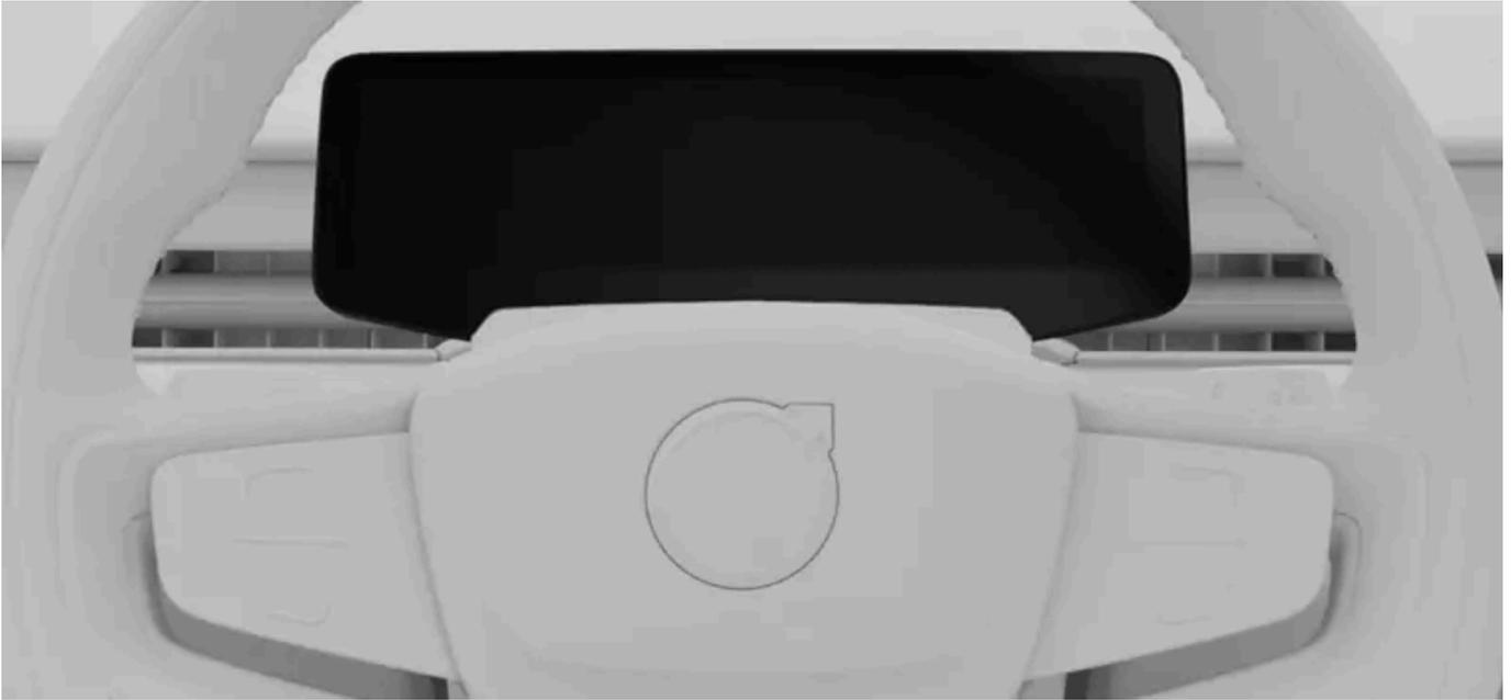
The driver display is located in front of the driver, behind the steering wheel. Its position changes along with the steering wheel when you adjust it to your preferred driving posture.
