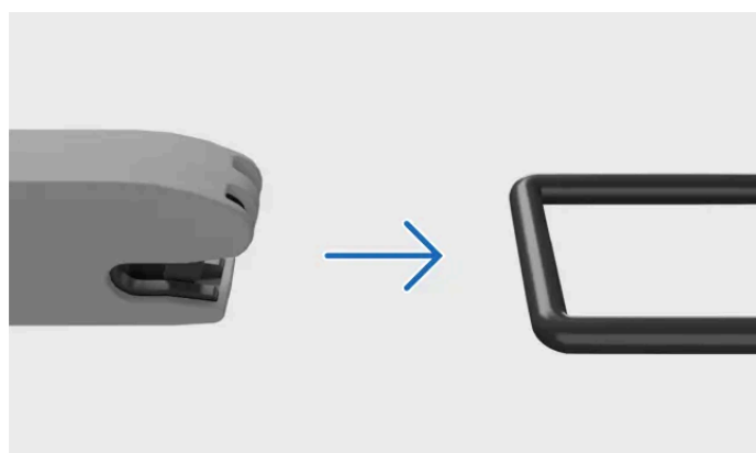
Attaching to ISOFIX anchorage point
