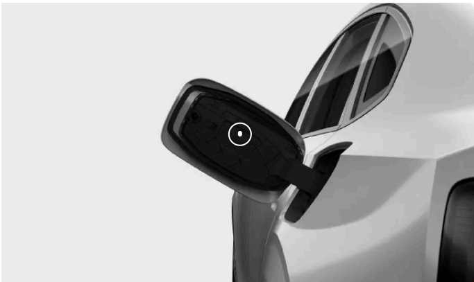
The identification label are located on the inside of the charging lid.
