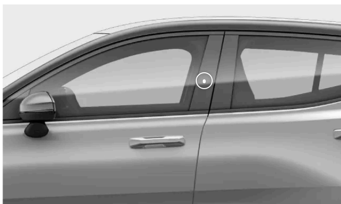
Key reading location on the door pillar
