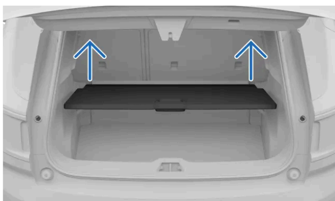
Illustrative guide for removing the cargo hatch.
