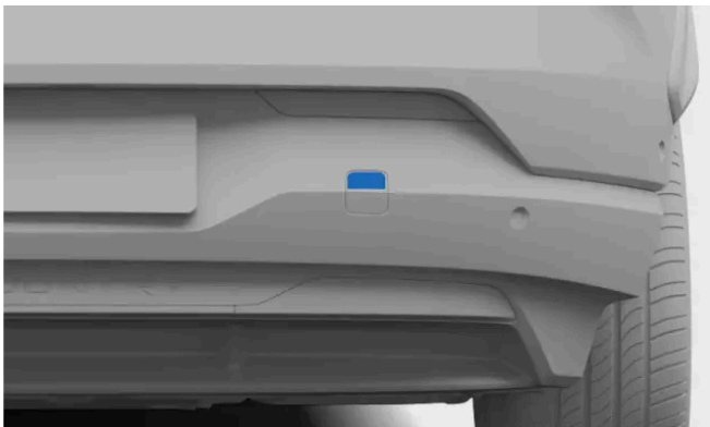
Rear towing eye fastening cover.
