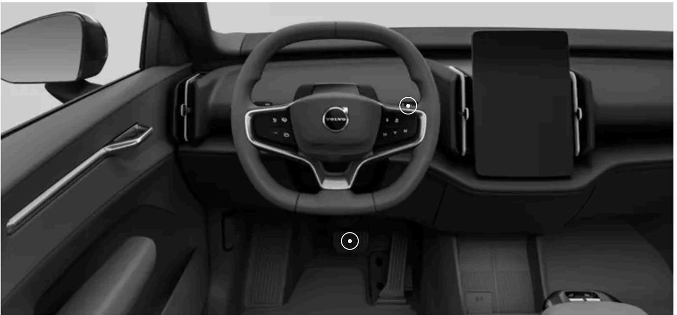
Your main interaction points for starting your car are the brake pedal and the gear stalk.
