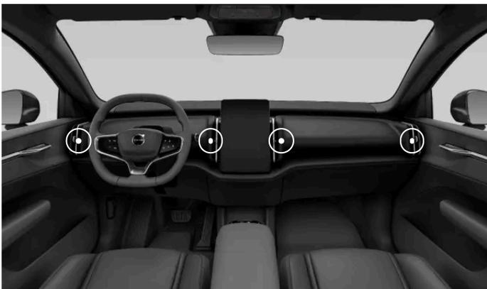
The positions of the adjustable air vents.
