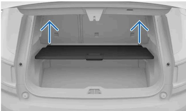
Illustrative guide for removing the cargo hatch.
