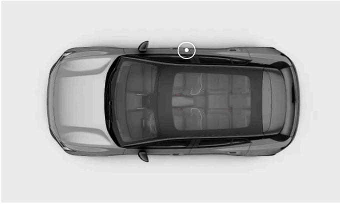
The product label is located on the right-hand door pillar and will be visible when the door is opened.
