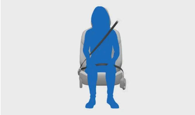
The seatbelt locks itself to act as a safety restraint under certain conditions. They include sudden and forceful pulling of the belt, if the car is driven aggressively and if the car is on a steep incline.
