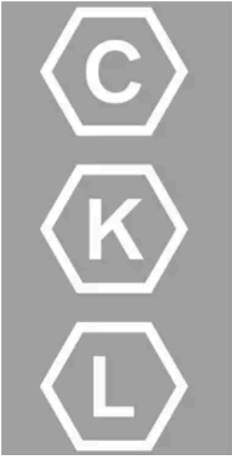
Charging compatibility identification labels.
