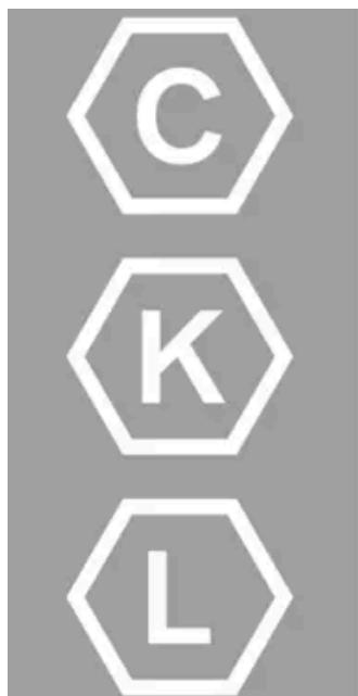
Charging compatibility identification labels.
