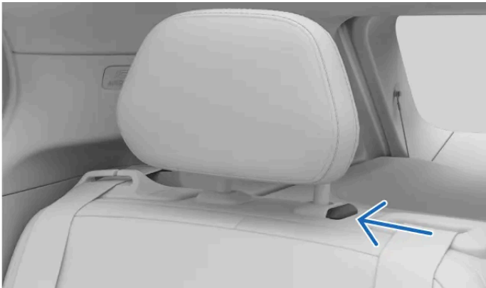
Locking button on the headrest
