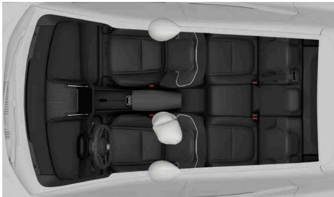
Side-on collision airbags for the front occupants.
