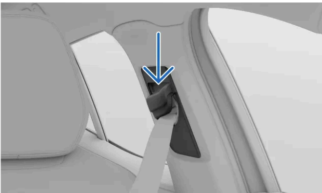
Seatbelt upper anchor point
