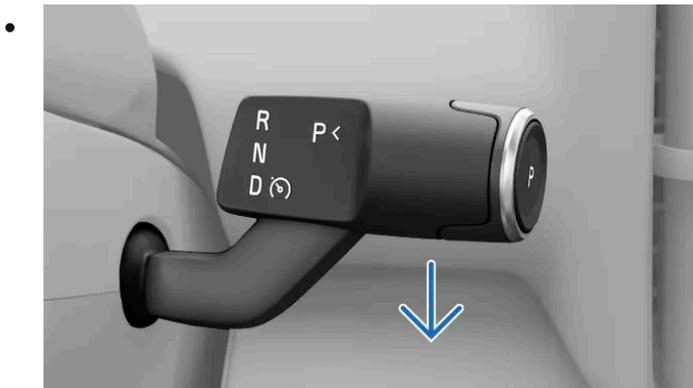
Pull the right-hand side steering wheel stalk all the way down.
