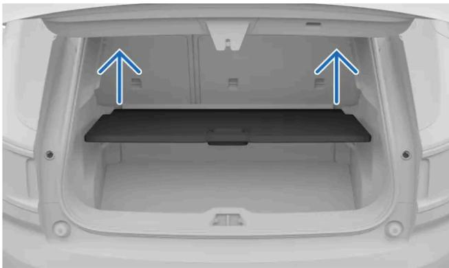
Illustrative guide for removing the cargo hatch.
