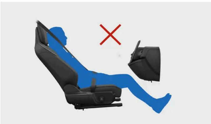
Do not fold the backrest to a lying position. The seatbelt must remain tensioned against the shoulder.
