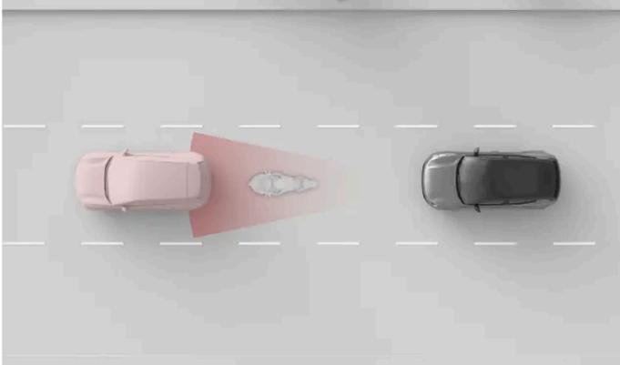
The smaller motorcycle and the car are close to each other and overlap, making detection of the motorcycle less accurate.
