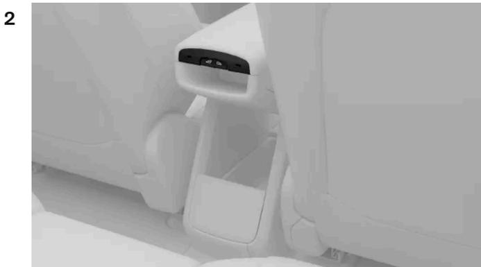
From the rear seats, you can operate the rear windows using the switches on the rear end of the centre armrest.
