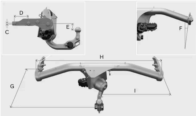
Dimensions, mounting points in millimetres (inches)
