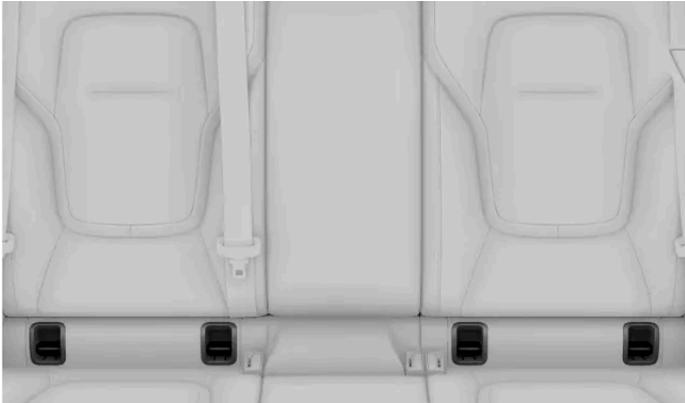
The ISOFIX anchorage points for the rear seats are located behind a flap in the lower part of the backrest on the outer rear seats. The flap needs to be unfolded to access the anchorage points behind it.
