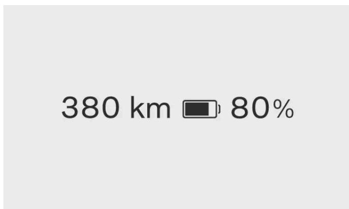
The battery meter is shown in the driver information area at all times. The battery icon's colour changes depending on the level of remaining charge in the battery.
