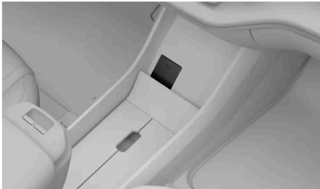
The location of the key card reader, used if you start the car with a key card or a discharged distance-capable key.
