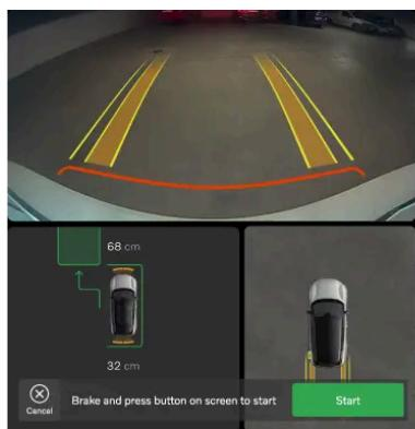
**2** To confirm the path and start the manoeuvre, press the **Start** button in the display.
