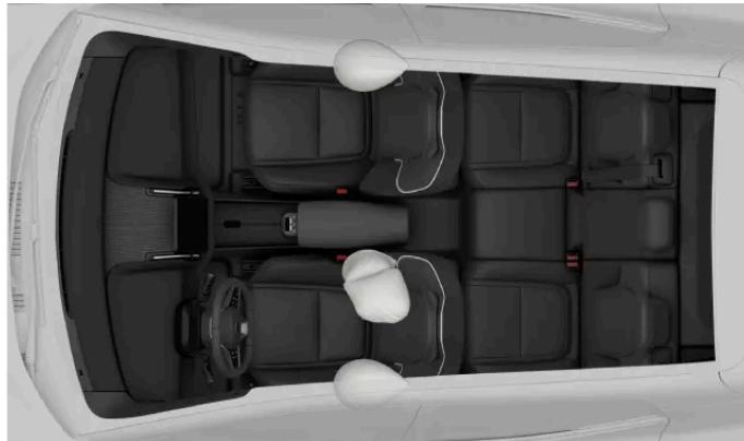
Side-on collision airbags for the front occupants.
