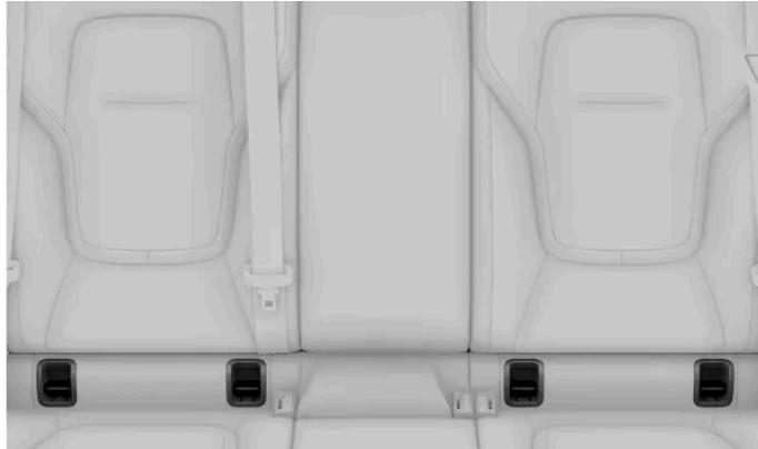
The ISOFIX anchorage points for the rear seats are located behind a flap in the lower part of the backrest on the outer rear seats. The flap needs to be unfolded to access the anchorage points behind it.
