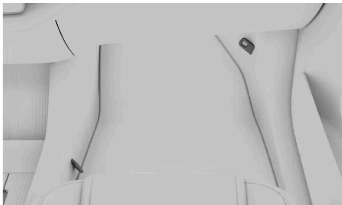
With the front lower tether accessory<sup>[1]</sup>, the anchorage points for the front passenger seat are located on the sides of the seat's footwell.
