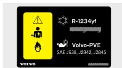
The label with information on climate system fluids is located under the bonnet, on the right-hand side of the car.
