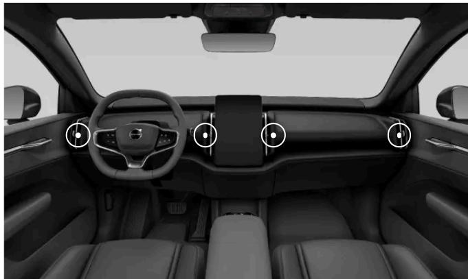
The positions of the adjustable air vents.
