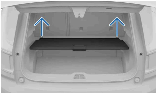
Illustrative guide for removing the cargo hatch.
