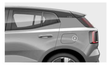
3 Remove any protective covers from the charging port and cable connector.
