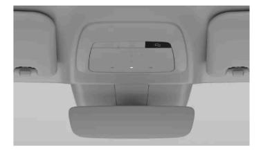
The assist button is located in the ceiling, on the right side of the overhead console.
