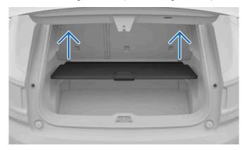
Illustrative guide for removing the cargo hatch.
