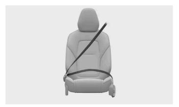
Correctly fastened and adjusted seatbelt.
