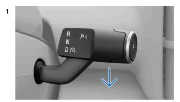
When appropriate, pull the right-hand steering wheel stalk all the way down.
