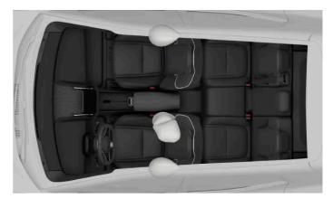
Side-on collision airbags for the front occupants.
