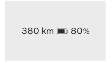
Your range is primarily related to your car's battery level and your driving practices but external conditions can also be a factor. The battery level and expected range are displayed in the driver information area. The expected range tells you how far you can drive with the current battery level. It is calculated based on your driving pattern, both current and historical, and on real-time driving conditions.
