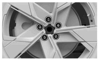
Tighten the wheel fasteners crosswise.
