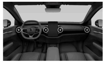
The positions of the adjustable air vents.
