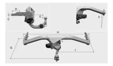
Dimensions, mounting points in millimetres (inches)
