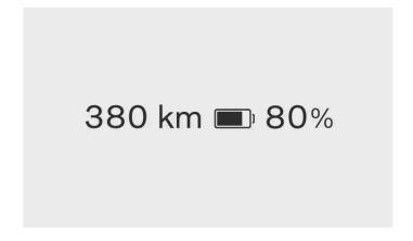
The battery meter is shown in the driver information area at all times. The battery icon's colour changes depending on the level of remaining charge in the battery.
