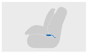
Child restraint installed using ISOFIX
