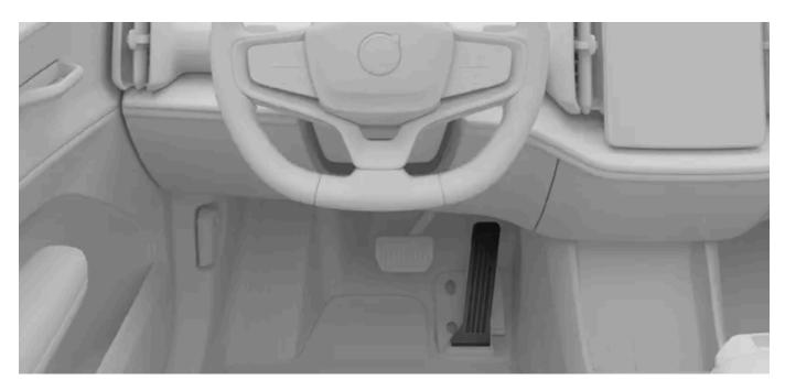
The braking behaviour changes through the use of the accelerator pedal. When you press the accelerator, the car accelerates as normal but releasing the pedal engages braking. The more you ease up on the pedal, the more braking action you get.
