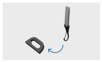
Fastening tether to lower tether anchorage point
