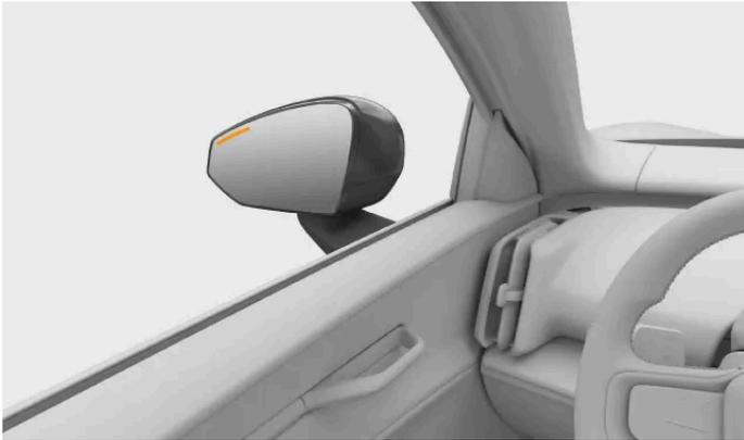
When the car detects traffic that is about to pass close to the car's sides, a light appears in the wing mirror along with a notification in the display. If you begin to open the door on the side of the detected traffic, the alert intensifies. A sound alert can occur along with the visual alerts depending on how urgent the warning is.
