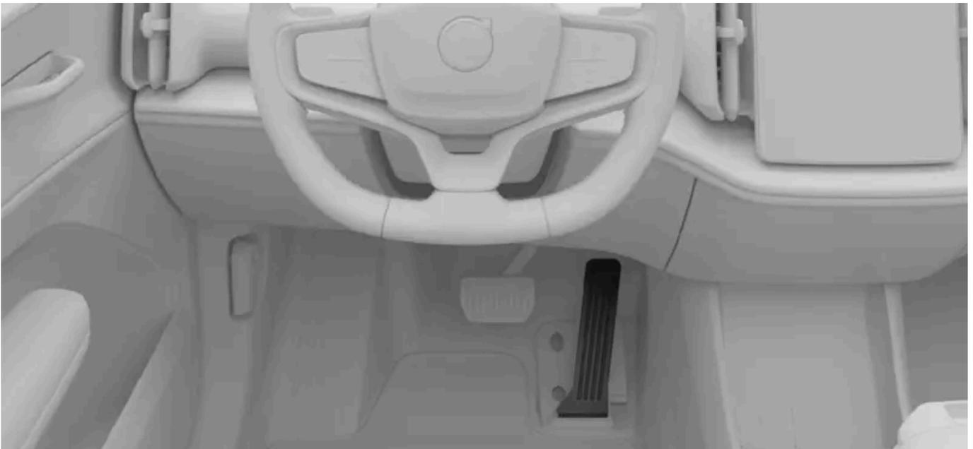
The braking behaviour changes through the use of the accelerator pedal. When you press the accelerator, the car accelerates as normal but releasing the pedal engages braking. The more you ease up on the pedal, the more braking action you get.
