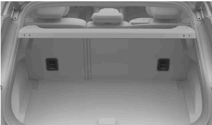
The top tether anchorage points for the rear seats are located on the back of the outer rear seats.
