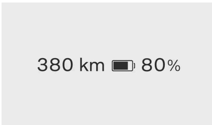
The battery meter is shown in the driver information area at all times. The battery symbol's colour changes depending on the level of remaining charge in the battery.
