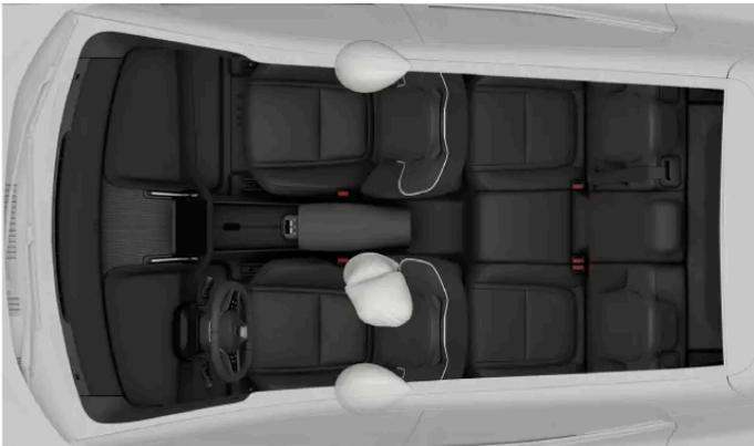
Side-on collision airbags for the front occupants.
