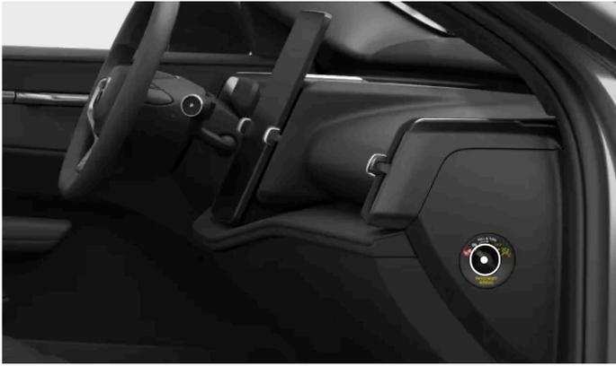
The airbag switch is located on the side of the dashboard and is accessible when the front passenger door is open.
