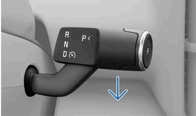
Pull the right-hand side steering wheel stalk all the way down.
