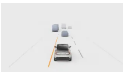
Warnings are indicated with a solid line marking in amber.
