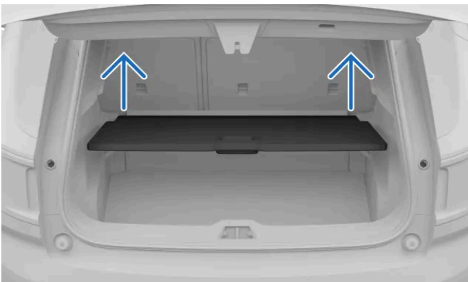
Illustrative guide for removing the cargo hatch.
