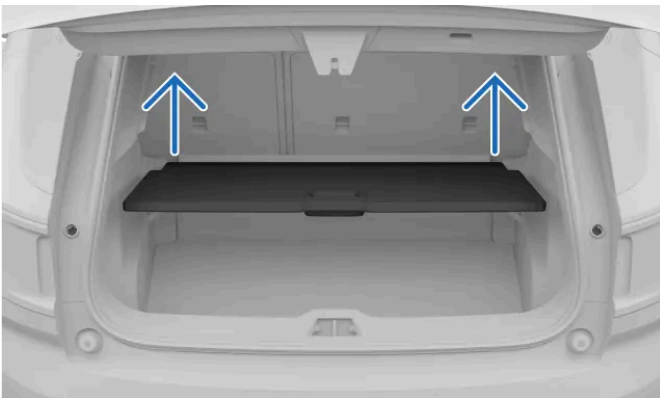
Illustrative guide for removing the cargo hatch.
