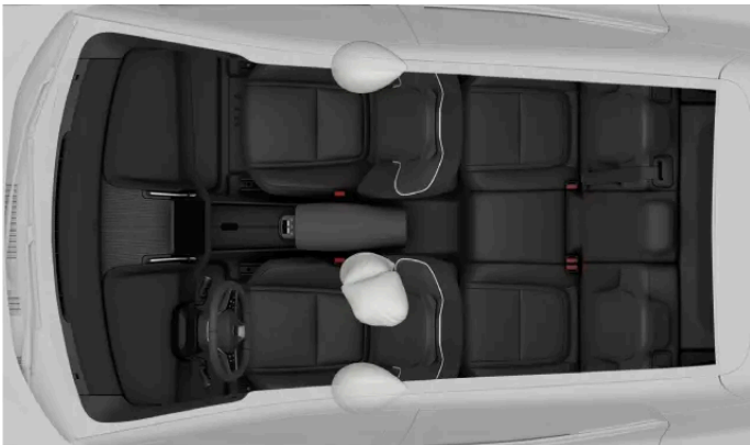
Side-on collision airbags for the front occupants.
