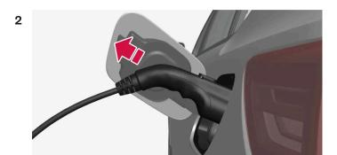
Unplug the charging cable from the car's charging input socket and close the hatch.
