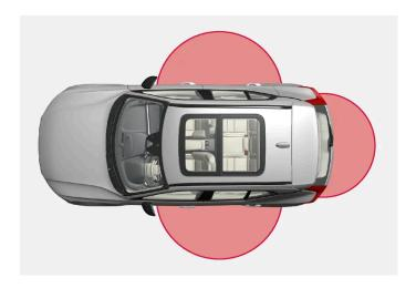
For keyless use, a key must be within a distance of approx. 1 to 1.5 metres (3 to 5 feet) from the car's doors or tailgate.
