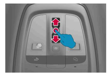
Make a smooth and continuous swiping motion backwards/forwards over the touch-sensitive control to fully open/close the panoramic roof. In the event of problems, try moving more quickly or more slowly.
