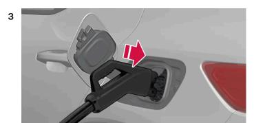
Grasp the charging cable with both hands and press the charging cable all the way into the car's charging input socket. Hold the charging handle upwards for several seconds. The charging cable is automatically locked into the charging input socket after a couple of seconds. Ensure that the charging cable is properly locked so that charging can start.
