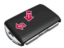
Refit the rear shell in reverse order to how it was removed. There is no logotype on the rear shell. Press in the shell until you hear a click, and then slide it the last few millimetres to its original position.
