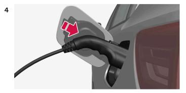
Remove the charging handle's protective cover and press the charging handle the whole way into the charging input socket.
