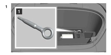
Take out the towing eye from the foam block under the bonnet.
