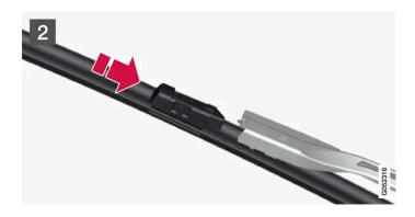
Make sure that the windscreen wipers are in service position and fold up the wiper arms. Service position is activated and deactivated via the centre display when the car is stationary and the windscreen wipers are not switched on.
