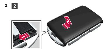
Slide the catch that was behind the front shell to the side, and slide the rear shell away from the key ring bracket.
