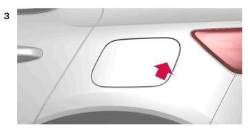
Press in the rear section of the cover to open the charging hatch [2].
