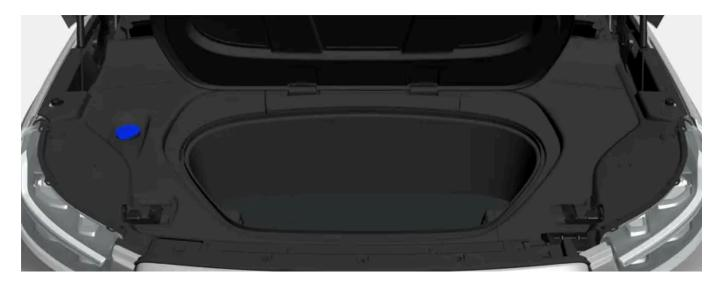
There is additional storage space under the bonnet. The car's towing eye and emergency puncture repair kit are also stored in the cargo area.
