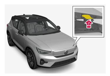
Move the handle under the bonnet upwards to release the catch and lift the bonnet.
