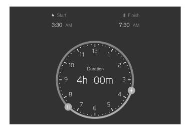
Select Charging → Set timer in the centre display and then activate the scheduling with Schedule charging. Use the controls at 4 and 11 to set the desired start and stop time for charging.
