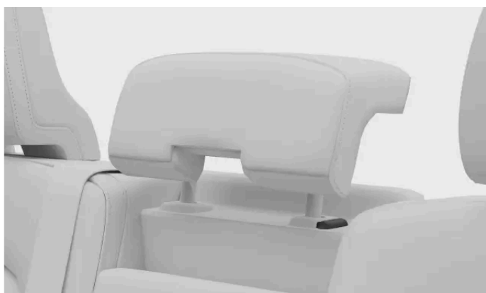
Locking button on the headrest
