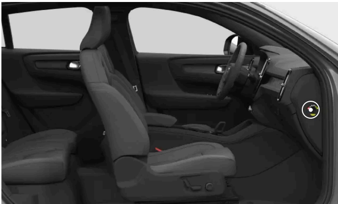
Location of the passenger airbag switch
