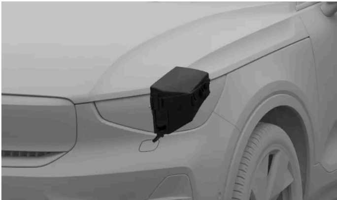
Fuse box location
