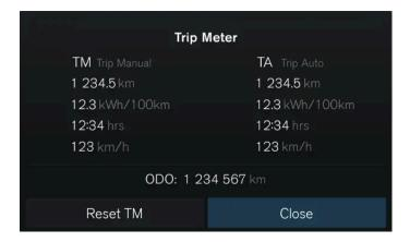
Your car has a trip meter and an odometer. The trip meter can show information on the car's driving distance and time, as well as your average driving speed.
