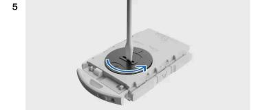
Using a suitable tool, such as a screwdriver or a coin, turn the battery cover anticlockwise to release it.
