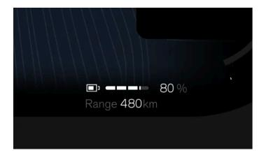
Your range is primarily related to your car's battery level and your driving practices but external conditions can also be a factor. The battery level and expected range are displayed in the driver display. The expected range is calculated based on your driving pattern, both current and historical.
