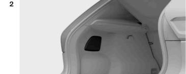
Press the top edge of the panel cover to make it pivot and remove it.
