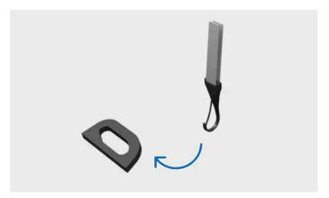
Fastening tether to lower tether anchorage point
