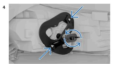
Unscrew the spring screw by turning anticlockwise. Leave the screw in the support bridge so that you can find it when you need it again.
