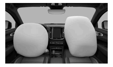
The driver side has two front airbags. The upper airbag is packed inside the steering wheel and the knee airbag is packed behind a panel below the steering wheel.
