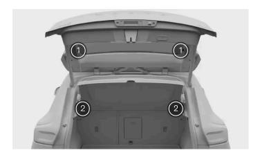
There are two attachment points on the parcel shelf itself and two on the boot hatch. When the parcel shelf is attached, cords run between attachment points on the parcel shelf and the boot hatch.
