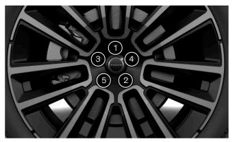
Tighten the wheel fasteners crosswise.
