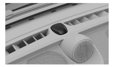
The alarm indicator is a light located in the centre of the dashboard, just in front of the windscreen. The indicator confirms when the alarm is enabled with a flashing red light.
