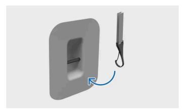
Fastening tether to top tether anchorage point
