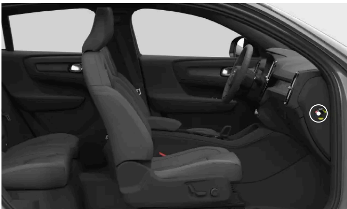
Location of the passenger airbag switch
