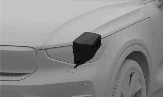
Fuse box location
