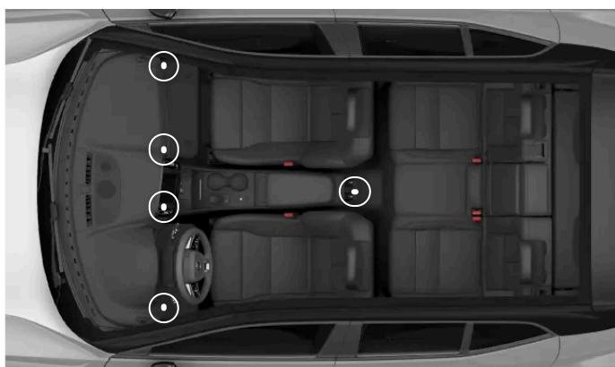
The locations of the adjustable air vents
