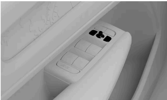
Controls for adjusting the wing mirrors
