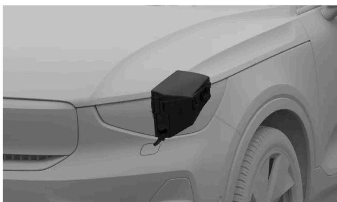
Fuse box location
