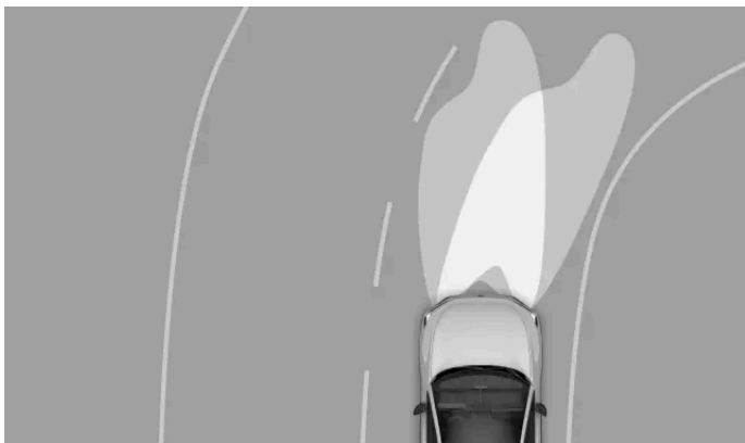
Typical function of the active bending lights
