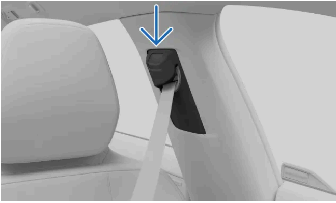
Seatbelt upper anchor point
