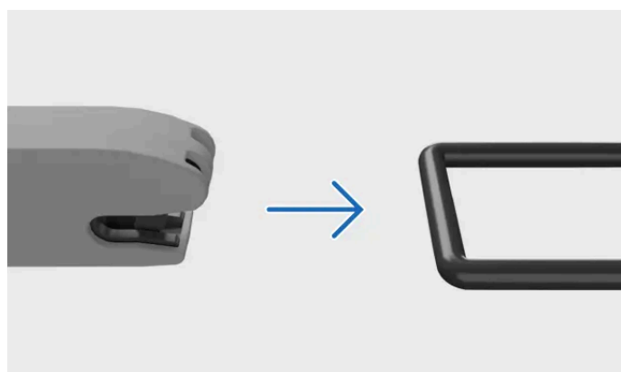
Attaching to ISOFIX anchorage point
