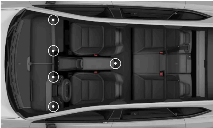
The positions of the adjustable air vents in the passenger compartment.
