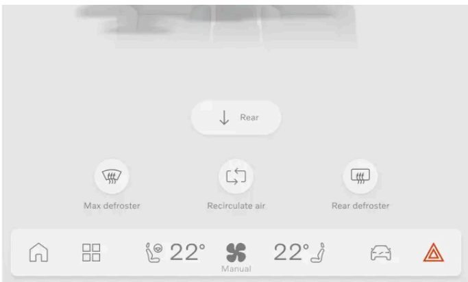
The location of the hazard lights button in the centre display
