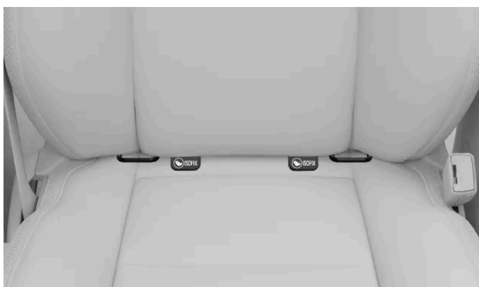
Locations of ISOFIX anchorage points for the front passenger seat
