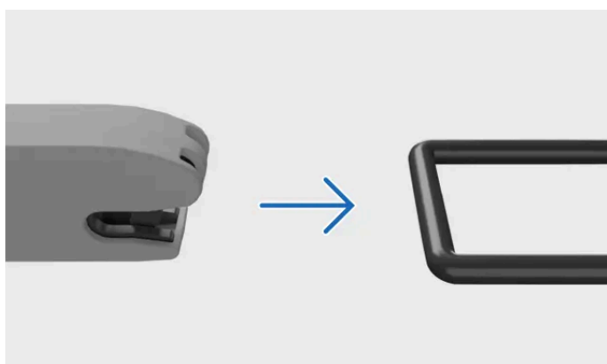
Attaching to ISOFIX anchorage point
