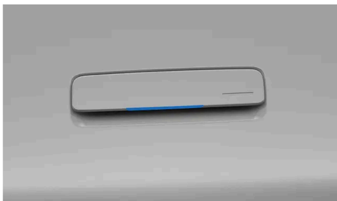
Touch point on the inner part of the door handle
