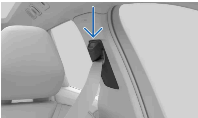
Seatbelt upper anchor point
