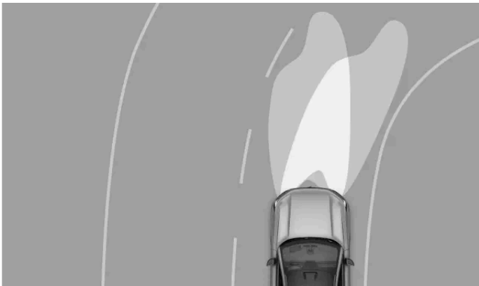
Typical function of the active bending lights.
