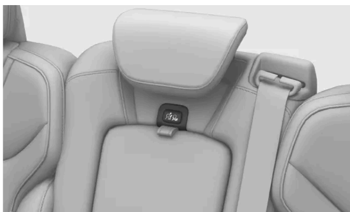
Locking button on the centre headrest
