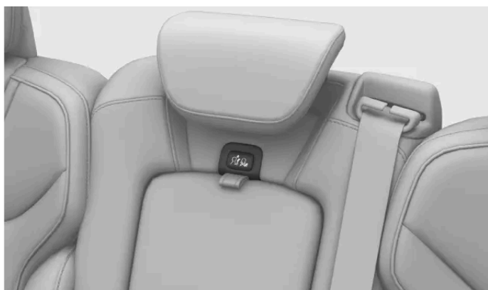
Locking button on the centre headrest
