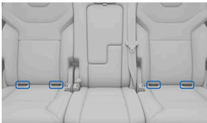
Locations of ISOFIX anchorage points for the second row seats
