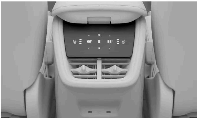
Climate controls in the tunnel console
