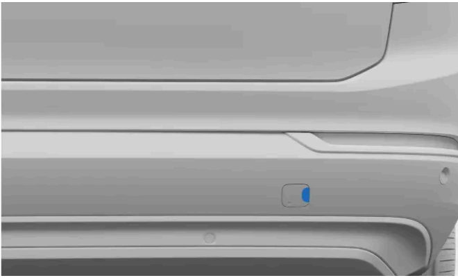
Rear towing eye fastening cover
