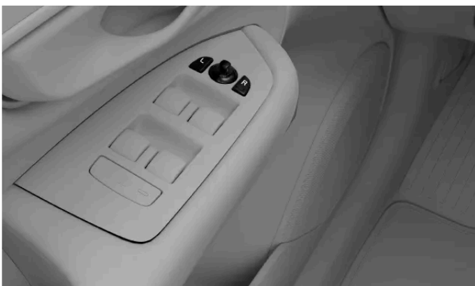
Controls for adjusting the wing mirrors
