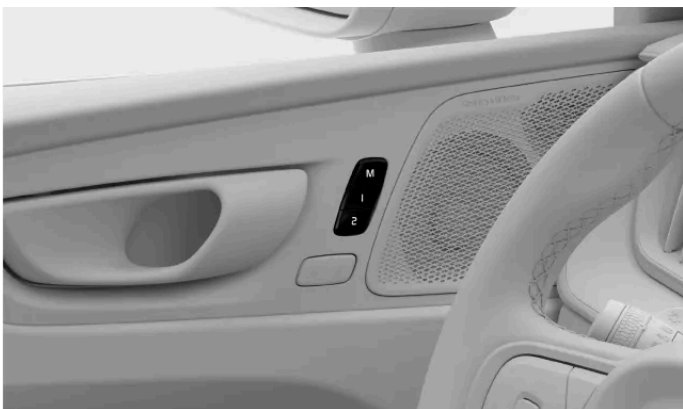
Location of the preset seat adjustment buttons
