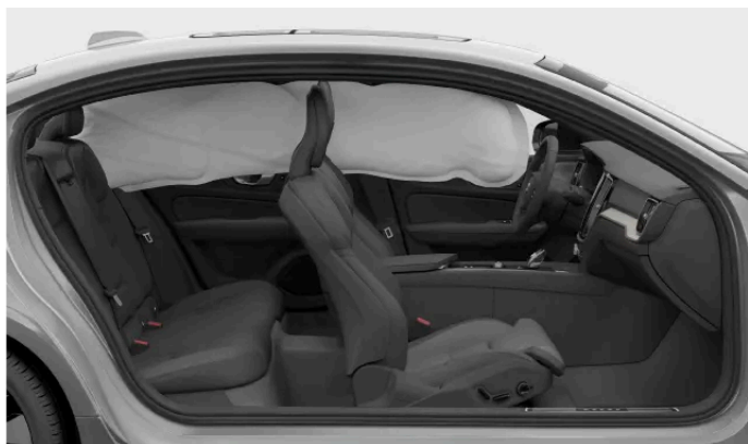
Inflatable curtain deployed on one side of the car.
