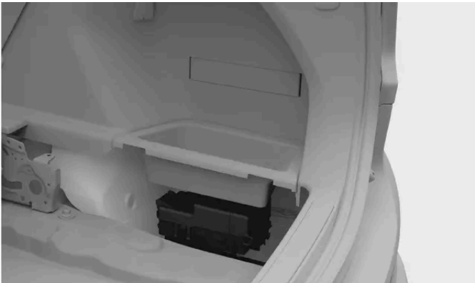
Fuse box location
