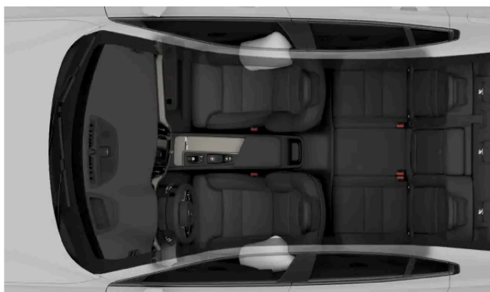
Side collision airbags for the front occupants.
