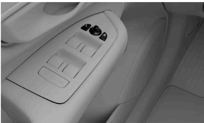
Controls for adjusting the wing mirrors
