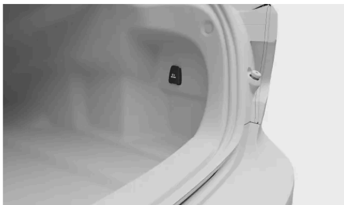
The 12 V electrical socket on the left-hand side in the boot
