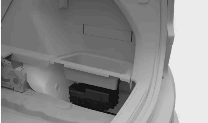
Fuse box location
