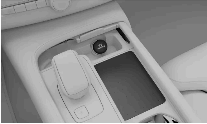
The 12 V socket in the tunnel console
