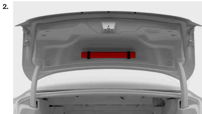
The warning triangle is secured with two clips on the inside of the boot hatch.
