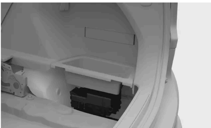
Fuse box location
