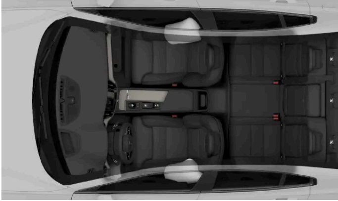
Side collision airbags for the front occupants.
