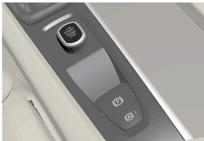
Start knob in the tunnel console.
