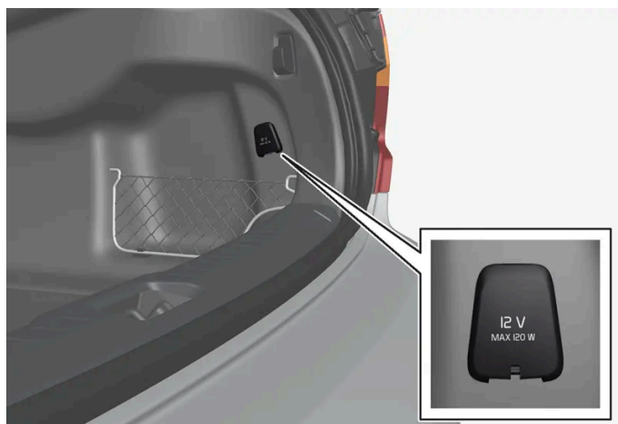
12 V electrical socket in cargo area*.
