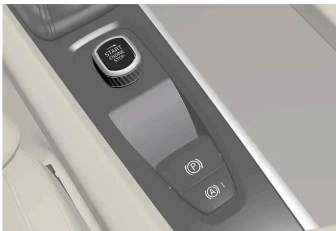
Start knob in the tunnel console.
