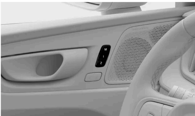
Location of the preset seat adjustment buttons
