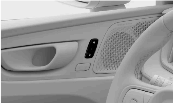
Location of the preset seat adjustment buttons
