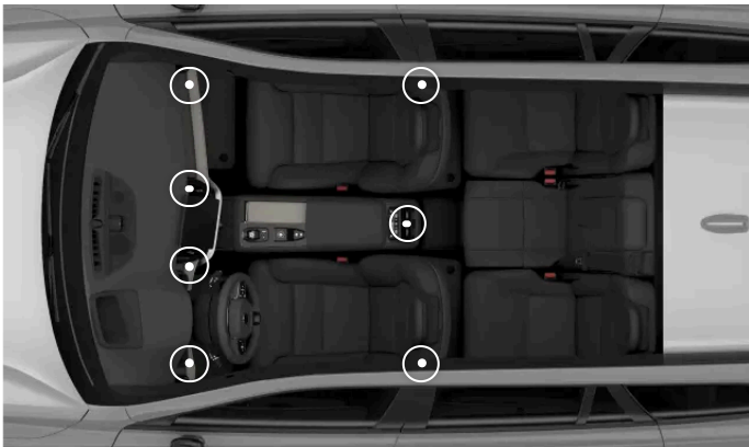
The locations of the adjustable air vents
