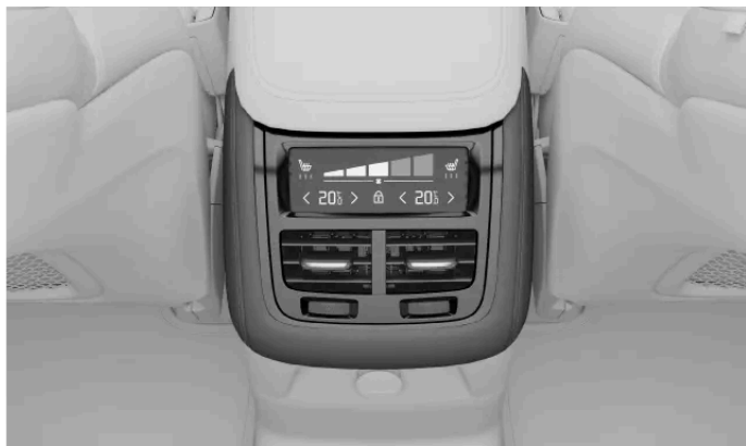
Climate controls in tunnel console
