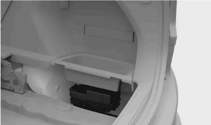
Fuse box location
