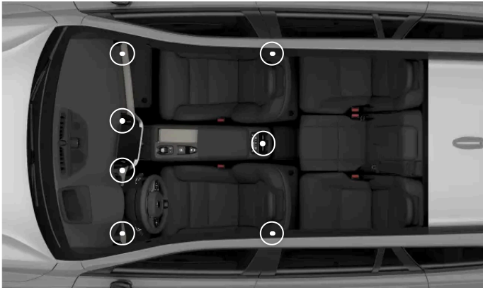
The locations of the adjustable air vents
