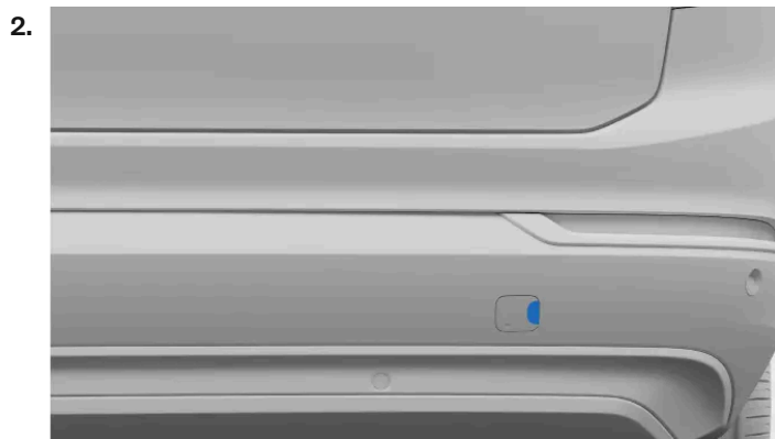
Rear towing eye fastening cover
