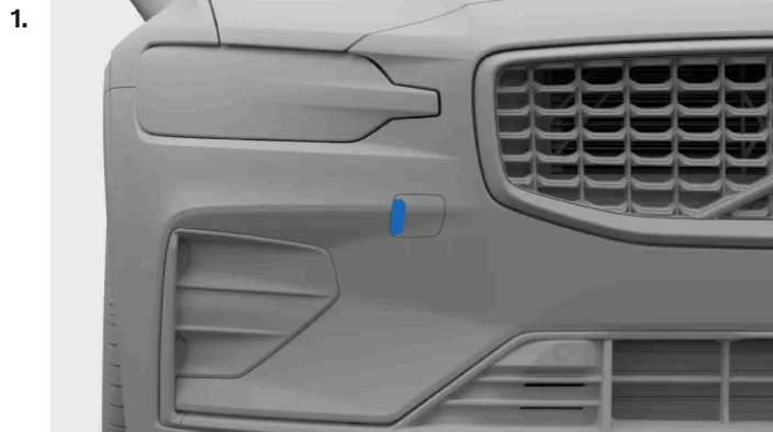
Front towing eye fastening cover
